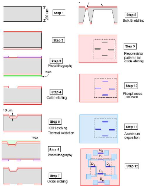
Steps to fabricate membrane for MEMS pressure sensor
