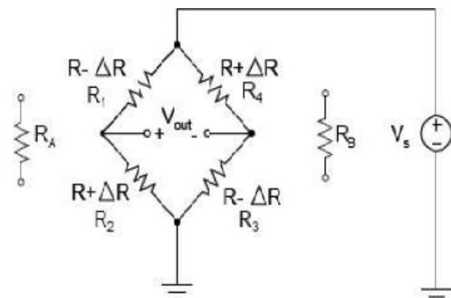
Fig. 1: Wheatstone bridge configuration of piezoresistors for pressure sensor. RA and RB are sensor resistors.
