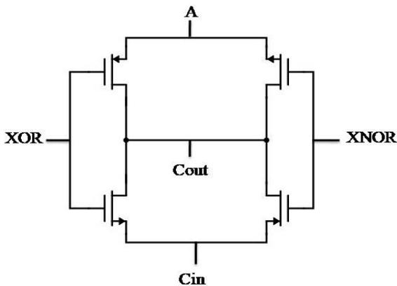
Fig. 4. Schematic structure of the carry generation module
