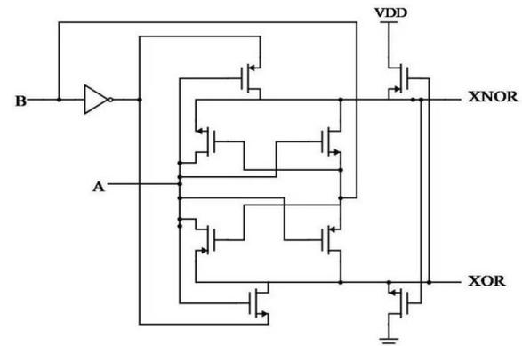
Fig. 2. Schematic structure of XOR-XNOR module
