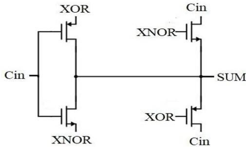
Fig. 3. Schematic structure of Sum generation module
