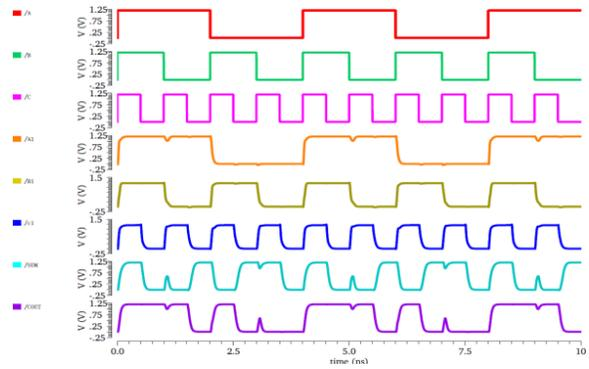
Fig. 5. Time-domain simulation results (waveform) of FA circuits
