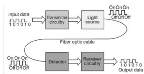
Fig.1. Basic fiber optic communication system
