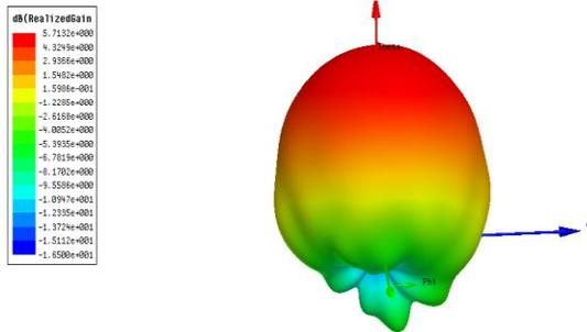
Figure 6. Patch 3D Radiation Pattern
