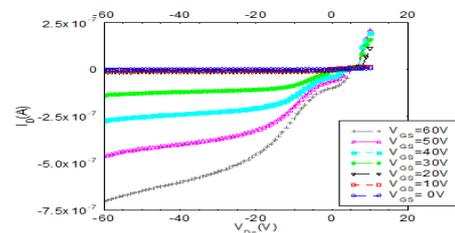
**Fig 2: I-V characteristics of Copper Thaloecyanine(CuPc) based Organic Thin Film Transister.**
