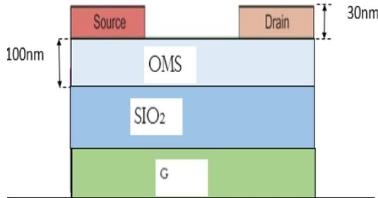
**Fig1: Schematic illustration of OTFTs dimension in side view.**
