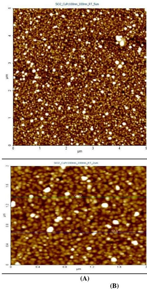
**Fig 3:**AFM topographic images of CuPc thin films grown at substrate temperature of 30 °C with thickness (A) 5μm and (B) 2μm
