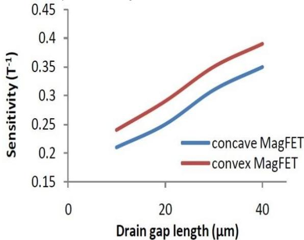
**Fig 3. Variation in Sensitivity with Drain gap length**
