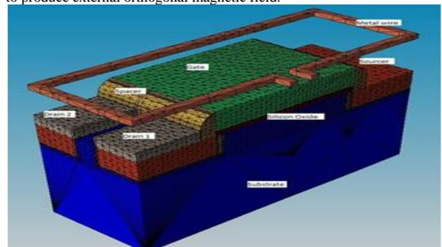
**Fig. 2 Geometrical Design of MagFET**
