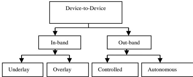
Fig. 2 Device-to-Device (D2D) Classification
