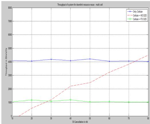
Fig. 11 Throughput Of System For Down-link Resource Reuse- Multi Cell
