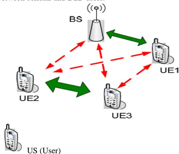
Fig. 1 Device-to-Device (D2D) Communications [1]
