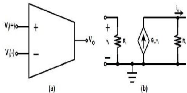
Fig 1. OTA Schematic Symbols and Equivalent Circuit
