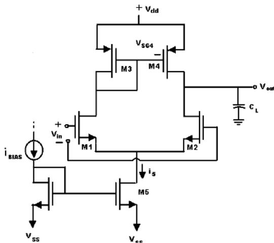
Fig 2. CMOS OTA Circuit
