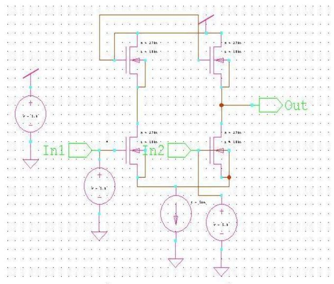
Fig 3. DC analysis current mirror circuit
