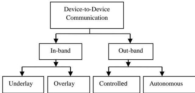
Fig. 2 Device-to-Device (D2D) Classification
