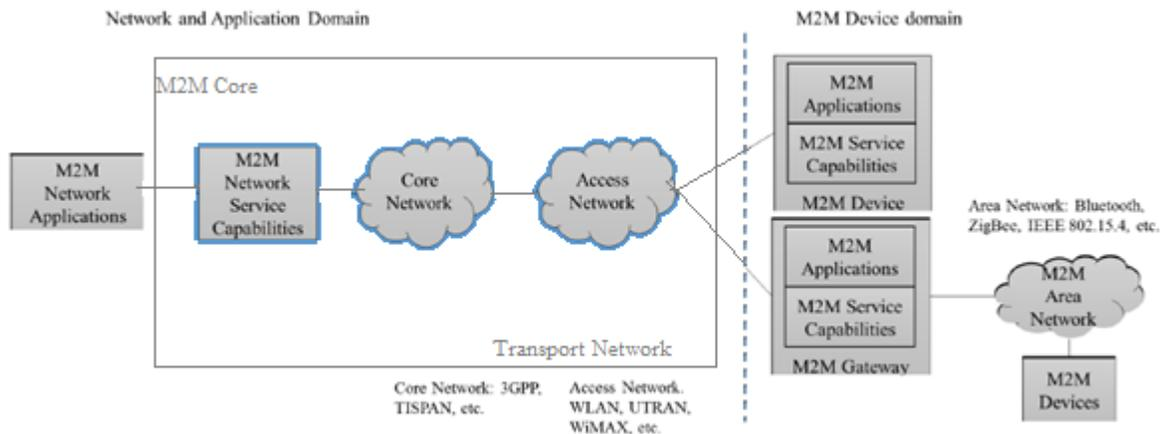
Fig. 4 European Telecommunications Standards Institute (ETSI) Machine-to-Machine (M2M) high level system overview [15]
