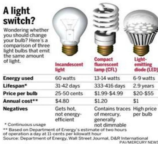
Fig. 2 Comparison of incandescent light lamps, Fluorescent lamps and LED lamps
