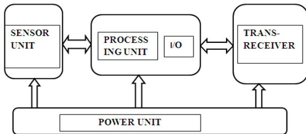
Fig. 2 Architecture of sensor node
