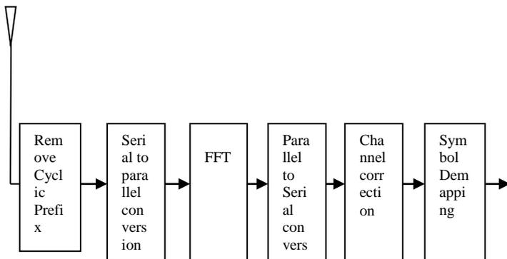
Fig. 2 Block diagram of OFDM Demodulator
