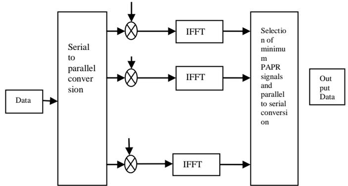
Fig. 3 Block diagram of selective mapping technique
