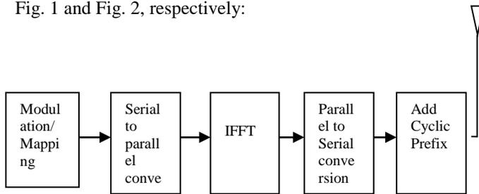
Fig. 1 Block diagram of OFDM Modulator
