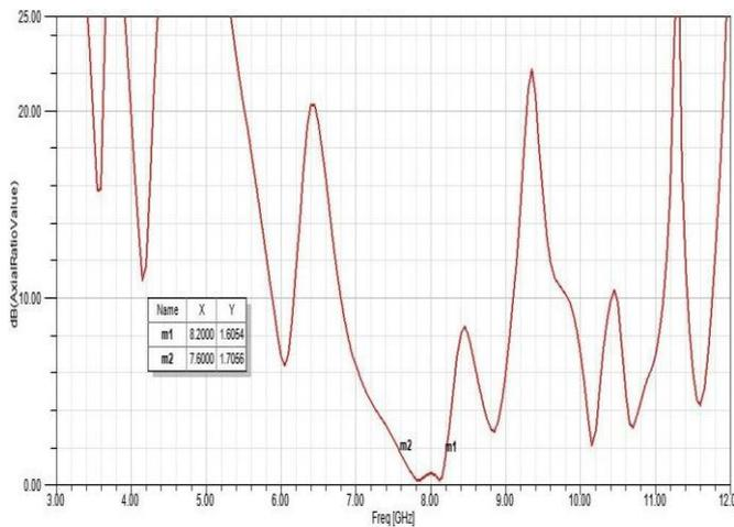
Fig 4(c): Axial Ratio of proposed MPA
