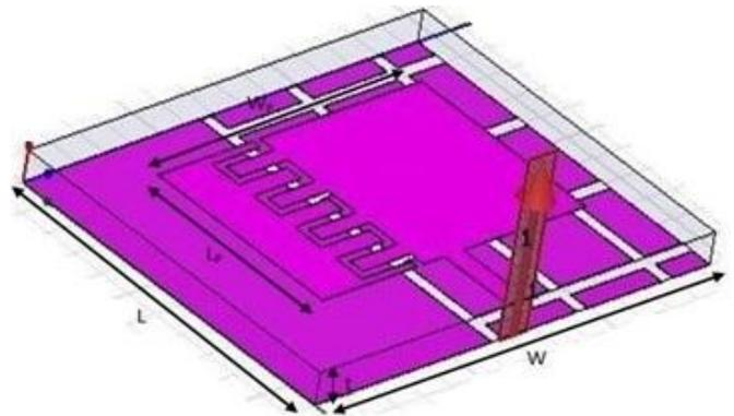
Fig 1: Schematic diagram of microwave-fed meander line loaded MPA placed over PDGS
