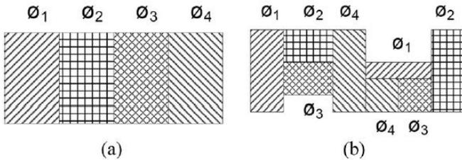
Fig 6. QCA clocking floorplans: (a) columnar Region and (b) zone Region.
