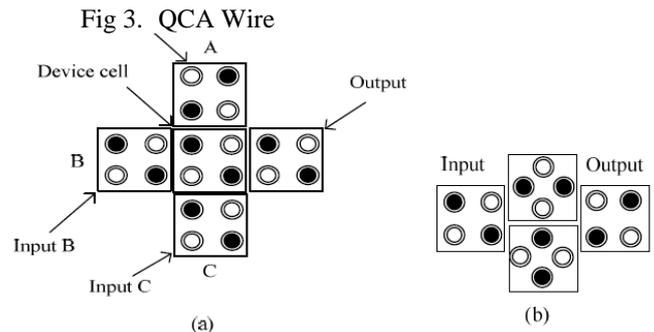
Fig 4. QCA (a) Majority Gate and, (b) Inverter
