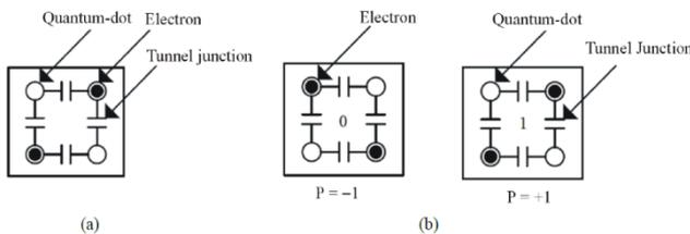
Fig 1. QCA Regular cell polarization
