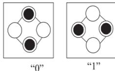
Fig 2. QCA Rotated Cell
