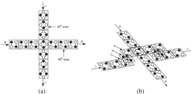
Fig 7. Crossovers in QCA: (a) Coplanar crossovers and, (b) Multilayer crossovers.
