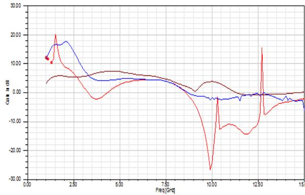
Fig.5. Gain Vs Frequency Curve of HMSA-PG (Red), HMSA-FS (Blue) and HMSA-CG (brown)
