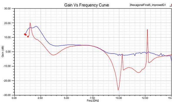
Fig. 2. Gain Vs Frequency Curve of conventional (Red) & modified HMSA (Blue)[11]
