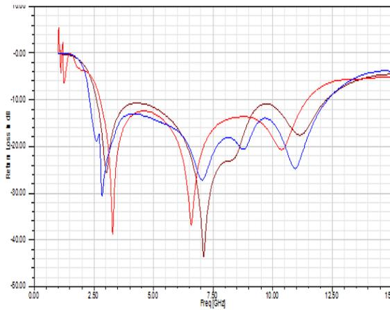
Fig. 4. Comparison of Return Loss of HMSA-PG (red), HMSA-FS (blue) and HMSA-CG (brown)
