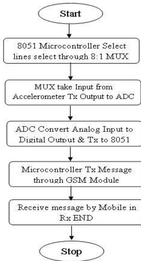
Figure: Flow Chart Accelerometer working
