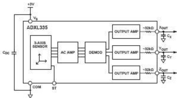
Figure 2: General Block Diagramme of Accelerometer
