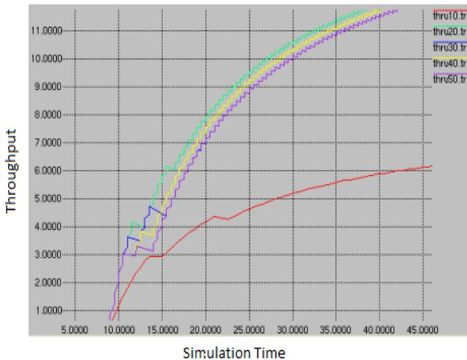
Fig.3. Throughput comparison for different speeds of mobile node with increased packet size
