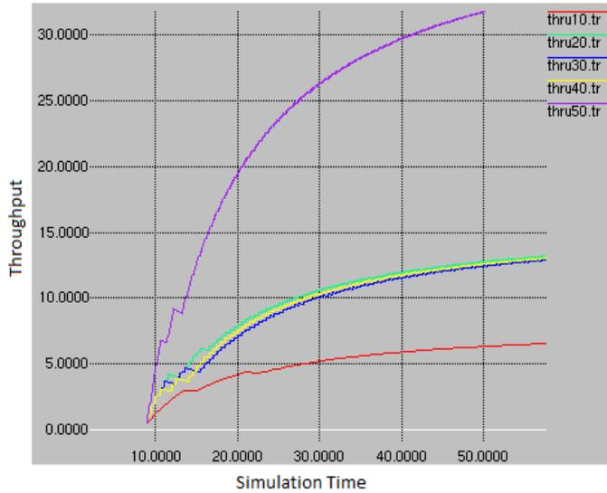
Fig.5 Throughput comparison for different speeds of mobile node with increased packet size and decreased interval
