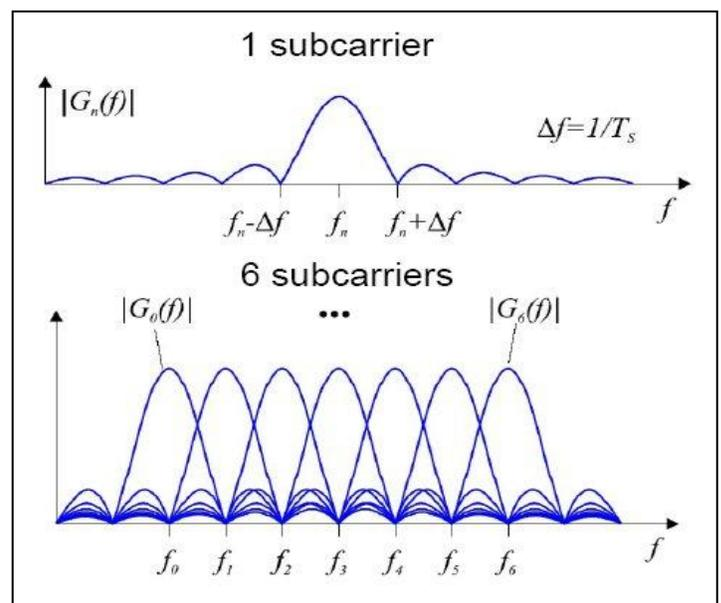
Fig 1. OFDM Subcarriers in Frequency Domain
