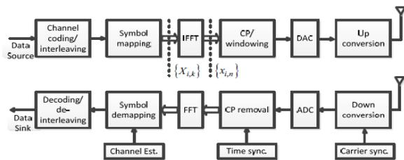
Fig. 4 Schematic of HF OFDM communication system
