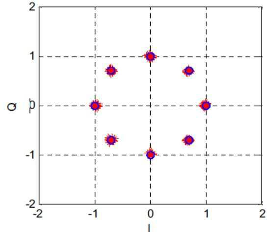
Fig. 6 The distribution of 8PSK constellation points after the clipping operation with 6dB PAPR threshold
