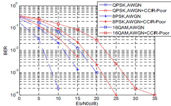
Fig. 7 Simulation of BER performance of the designed HF OFDM communication system
