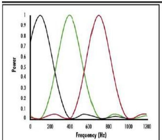
Fig. 2 Orthogonality of sub-carriers
