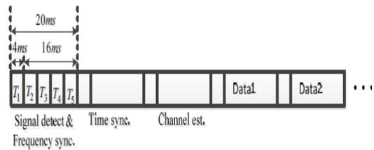
Fig. 5 Desired HF OFDM frame Structure
