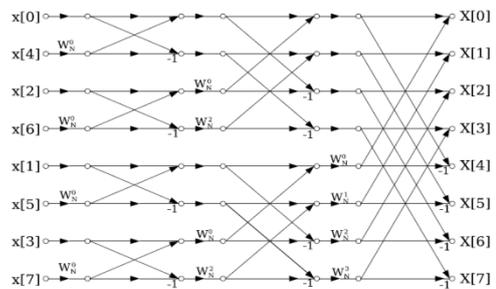
Fig. 3 Eight-point decimation-in- time FFT algorithm
