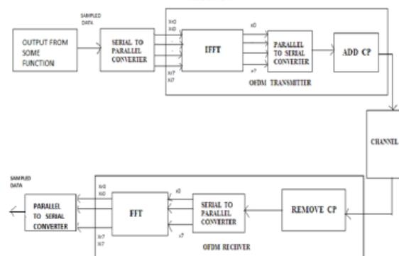
Fig. 1 Block diagram of conventional OFDM
