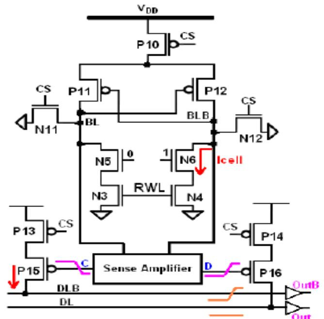
Figure 2 10T SRAM Cell
