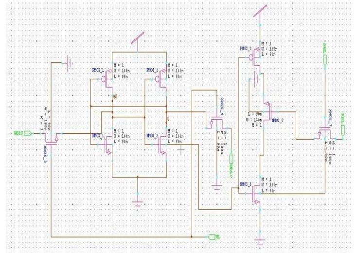
Figure 3 Schematic of 10T SRAM
