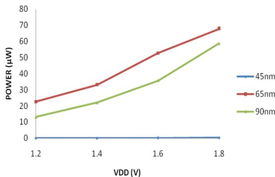
Figure 5 Variation of power with respect to Vdd
