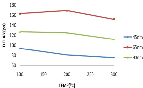
**Figure 8** Variation of Delay with respect to Temperature
