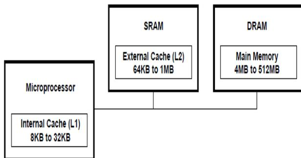
Figure 1 Typical PC microprocessor memory Configuration
