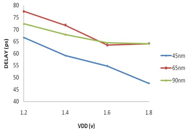
Figure 6 Variation of Delay with respect to Vdd
