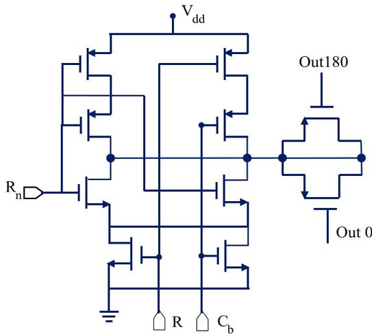
(a) Schematic of odd row of local decoder and varactor cell in varactor array.
