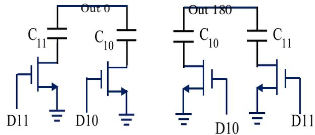
Fig.2. Detail of MIM capacitors implementation in proposed DCO.
