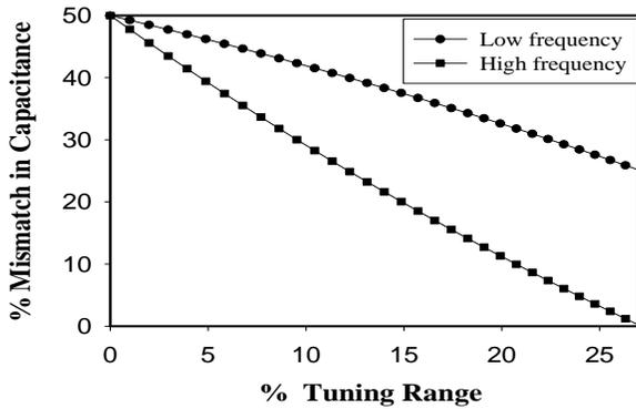
Fig.1. Optimization curve between tuning range and mismatch capacitance for DNL=0.5 LSB.
