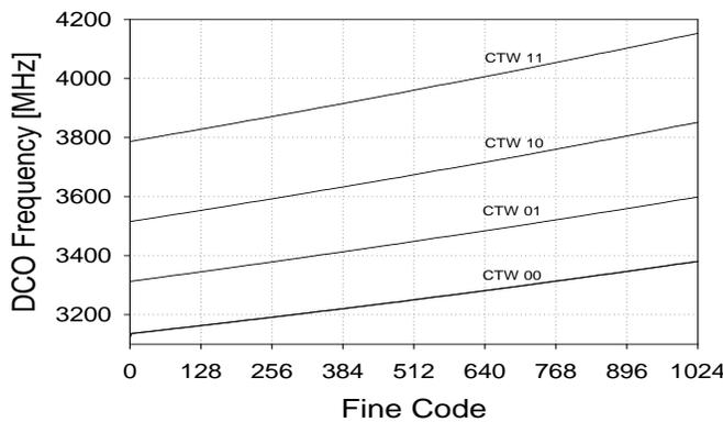
Fig.4.Simulated tuning range for CTW=(00)<sub>2</sub>, CTW (01)<sub>2</sub>, CTW (10)<sub>2</sub> and CTW (11)<sub>2</sub>.
