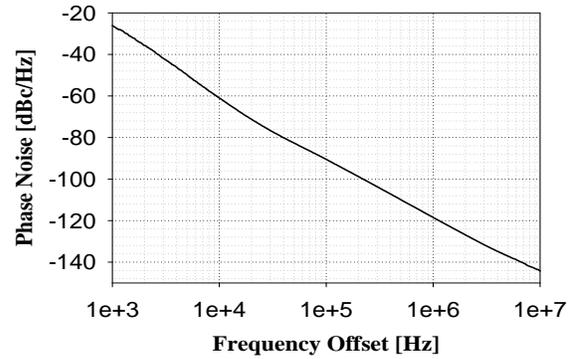
Fig.5. Simulated phase noise of proposed DCO.  $f_{osc}=3.8$  GHz, CTW=(11)<sub>2</sub>.
