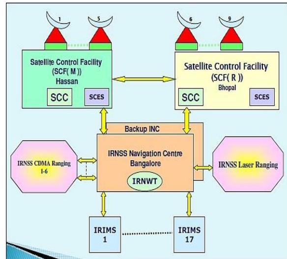
Fig. 5 IRNSS Ground Segment Architecture
