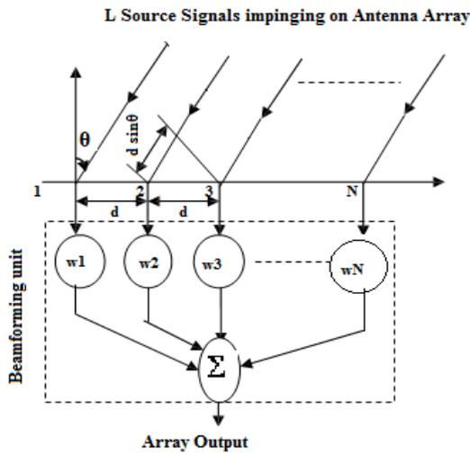
Fig. 1: Structure of Uniform Antenna Array with Beamforming Network.
