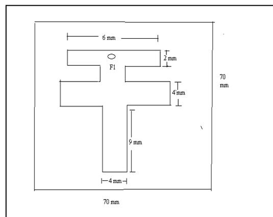
Fig.2: Geometry of the proposed first iterated T-shape slotted antenna
