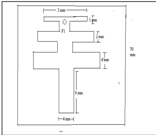
Fig.3: Geometry of the proposed second iterated T-shape slotted antenna
