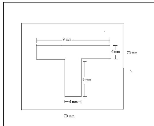
Fig.1: Geometry of the proposed T-shape slotted antenna
