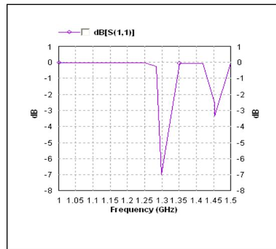
Fig.4: Simulated return loss for T-shape slot antenna
