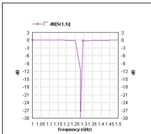
Fig.8: Simulated return loss for second iterated T-shape slot antenna
