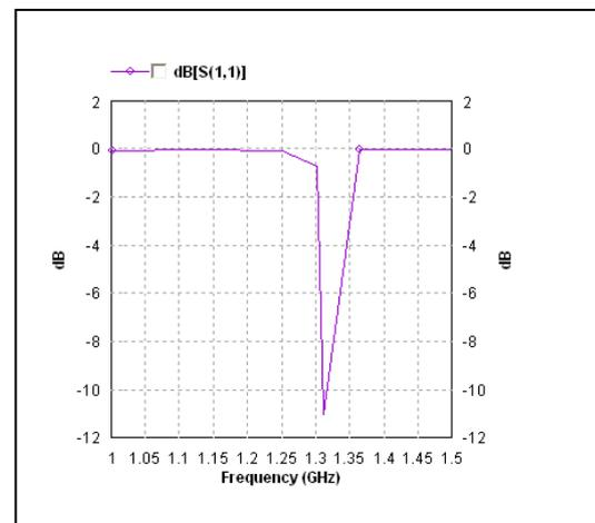
Fig.5: Simulated return loss for first iterated T-shape slot antenna
