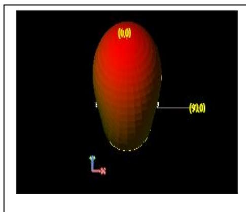
Fig.7: Simulated 3-D radiation pattern for first iterated T-shape slot antenna
