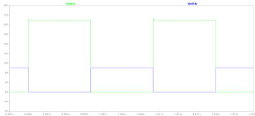
**Fig 7: Waveforms ( $V_{DC}$  (Green) and  $V_{GS}$  (Blue)) at 50Hz**
