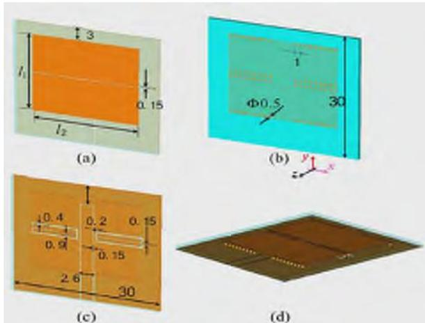
**Fig. 2: Geometry of the SRR-based antenna. (a) Top surface. (b) Midlayer. (c) Bottom surface. (d) The overall topology of the antenna (unit: mm) [38]**
