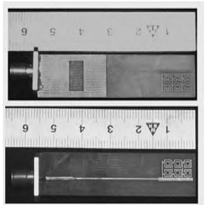
**Fig. 7:** Configurations of the proposed CP patch antenna loaded with the mushroom-like structure and the RIS. [43]
