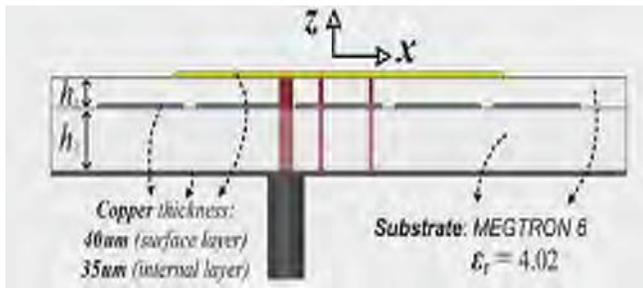
**Fig. 8: Geometry of the miniaturized patch antenna [45].**
