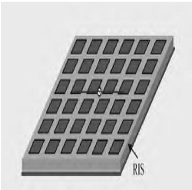
**Fig. 1: RIS is a 6X6 finite array of square patches printed on the PEC-backed dielectric material [31]**
