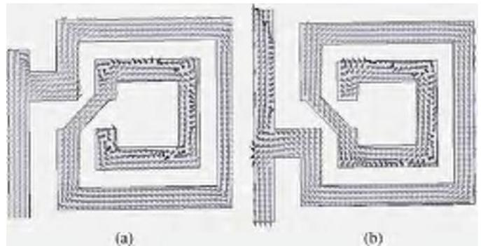
**Fig. 4: Surface Eigen current distribution on the (a) front and (b) back side of One unit cell [39].**
