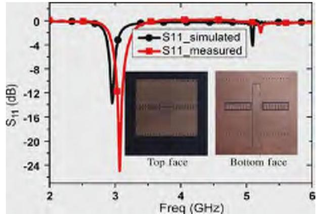
**Fig. 3: Simulated and measured S11 parameters of the improved SRR-based Antenna structure [38].**
