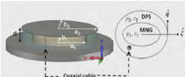
**Fig. 5:** A broadband planar antenna is proposed by loading a narrowband dipole antenna with six LHM unit cells [39].
