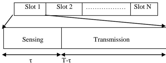
Figure 1- Frame structure for periodic spectrum sensing, where  $\tau$  denotes the sensing period and  $T - \tau$  denotes the data transmission or silent period.
