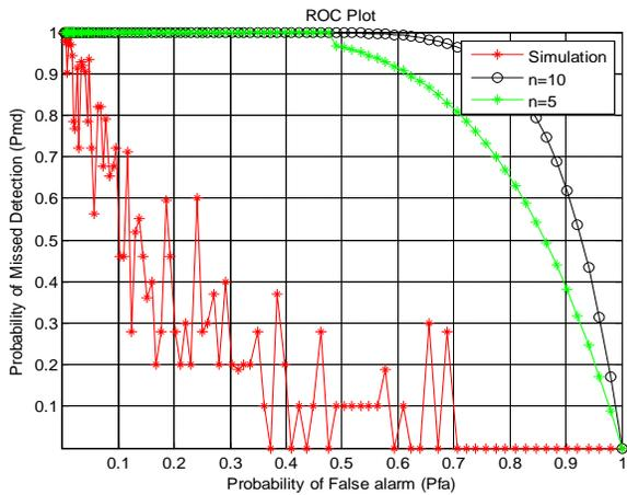
Fig 3. ROC curve for AND rule with the direct link over Rayleigh fading channel.
