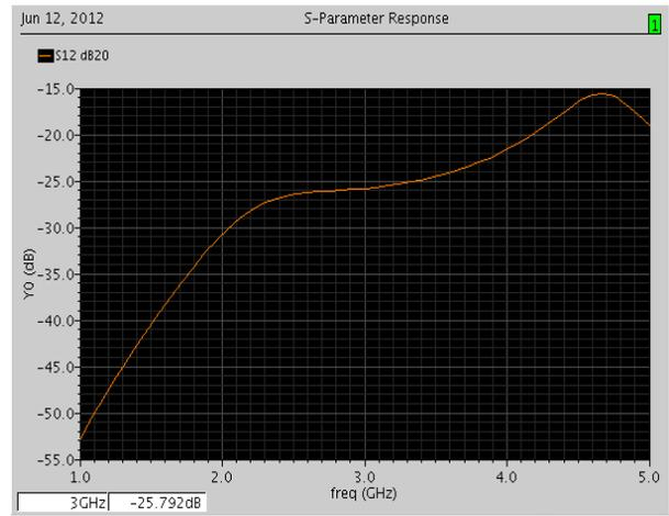
**Fig. 12: LNA Reverse power gain simulation result**
