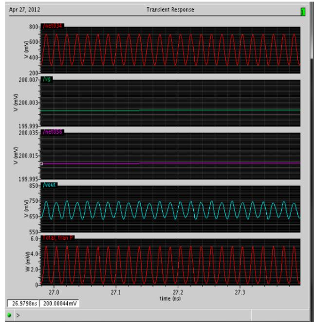
Fig. 16: Super-regenerative receiver output
