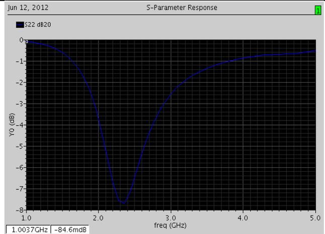
**Fig. 11: LNA outport reflection coefficient simulation result**
