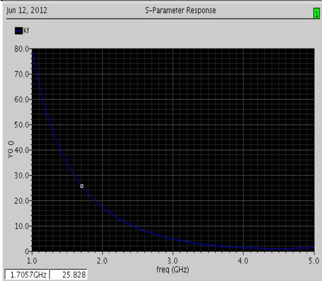
**Fig. 9: LNA small signal stability simulation result.**
