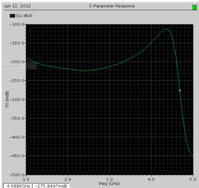
**Fig. 10: LNA input port reflection coefficient simulation result.**
