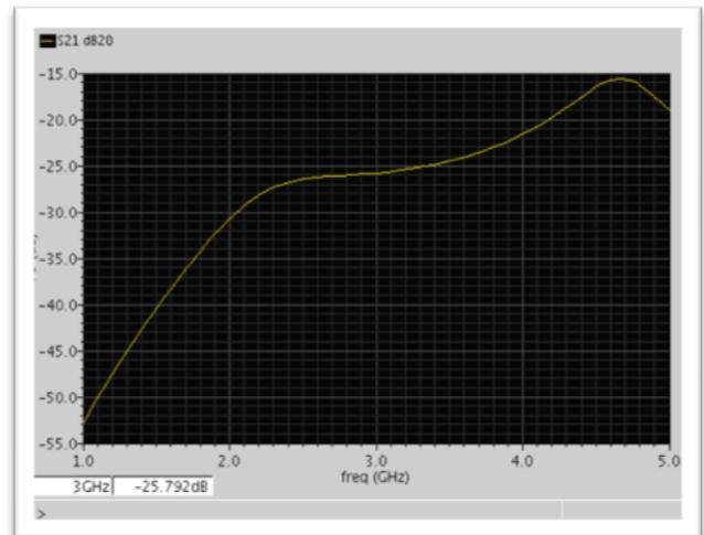
**Fig. 13: LNA Forward power gain simulation result**
