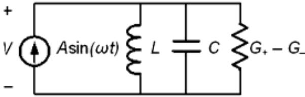
**Fig. 2: Parallel resonant circuit representing an SRO [3]**
